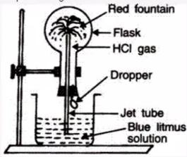
It happens because water introduced from dropper completely absorbs HCl gas, thereby creating a very low pressure within the flask. To make up for this loss in pressure, blue litmus solution rises in the jet tube and colour of litmus changes to red.
