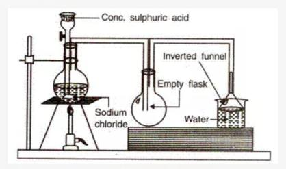
Hydrogen chloride gas prepared by the reaction of sodium chloride and sulphuric acid, is passed to inverted funnel arrangement through empty flask. An inverted funnel connected to the HCl gas supply is placed in a beaker in such a way that the rim of the funnel just touches the surface of water in the beaker. HCl gas coming through delivery tube fills the mouth of the funnel and then dissolves in water. By this way we get hydrochloric acid in the beaker.
